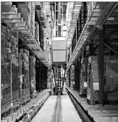
Warehouse robot. In the US, fully automated warehouses are becoming a reality as the industry is looking to reduce labor costs and improve productivity and accuracy.
